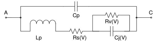
Figure 4 Small-signal Schottky diode model.  $C_p$  parasitic capacitance,  $L_p$  parasitic inductance,  $R_s(V)$  parasitic series resistance,  $R_v(V)$  video junction resistance,  $C_j(V)$  junction capacitance.
